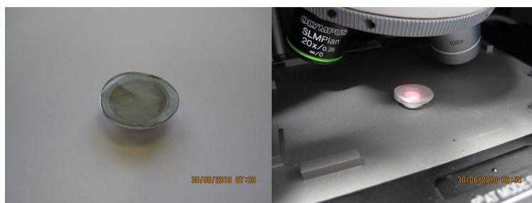
Figure 1: Mannitol prepared in covered sample holder (picture on the left) and Raman measurement of the sample via a RXN1-Workstation coupling (Kaiser Optical Systems Ltd., picture on the right).
